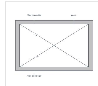
A nominally rectangular pane must be contained within a rectangle with sides having the permitted maximum and minimum dimensions.
